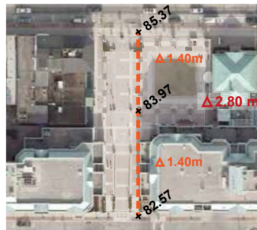
There is a significant grade change from north to south. From Lakeshore down to Robinson, the grade change is 2.80m. From Lakeshore down to the lower bowl area, the grade change is 1.40m.
