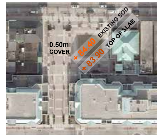
The entire Square lies above a parking structure. This is why existing tree pits are in raised planters. The approximate depth of cover in the lower bowl area is 0.50m.
