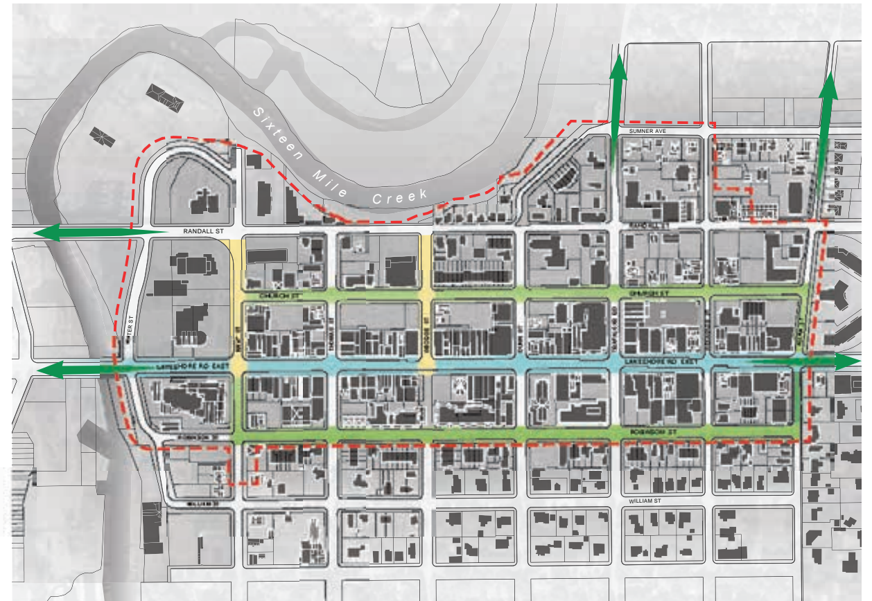
Dedicated buffered bike lanes on Church & Robinson Streets and sharrows on Lakeshore Road provide options for cyclists in the downtown. The ATMP will link downtown's cycling network to the broader town network via Randall, Lakeshore, Trafalgar and Allan, as shown.
