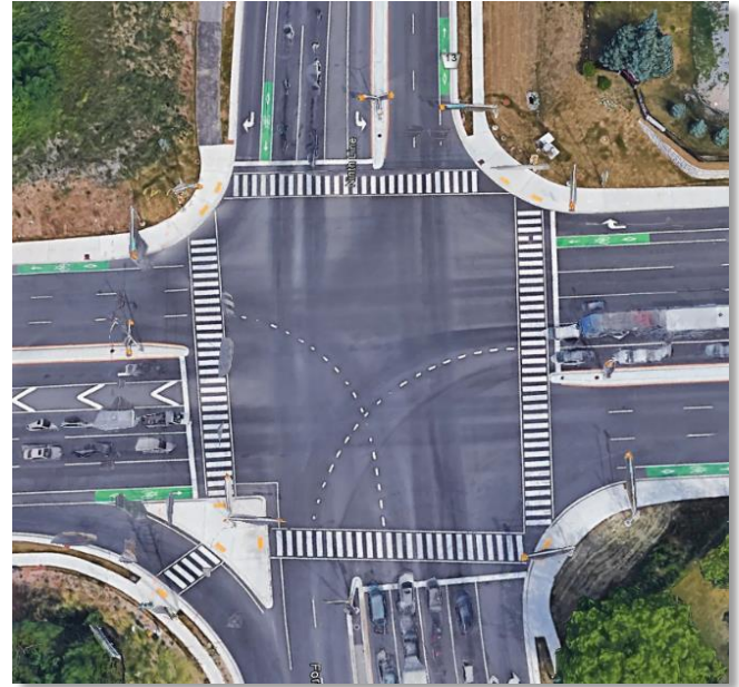
Figure 3- Example of Pavement Markings at intersection of Ninth Line / Ford Drive and Upper Middle Road E.
