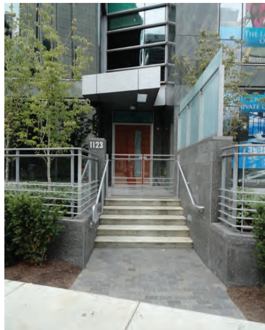
Slightly raised units provide for greater separation and privacy
