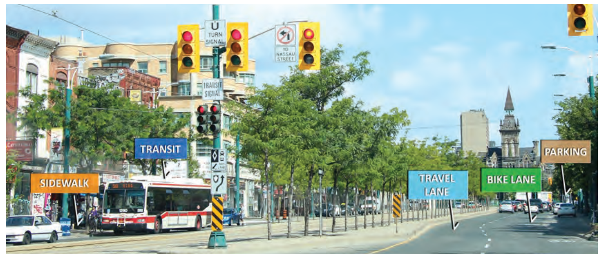
A complete street supports multiple travel modes: driving, transit, walking and cycling
