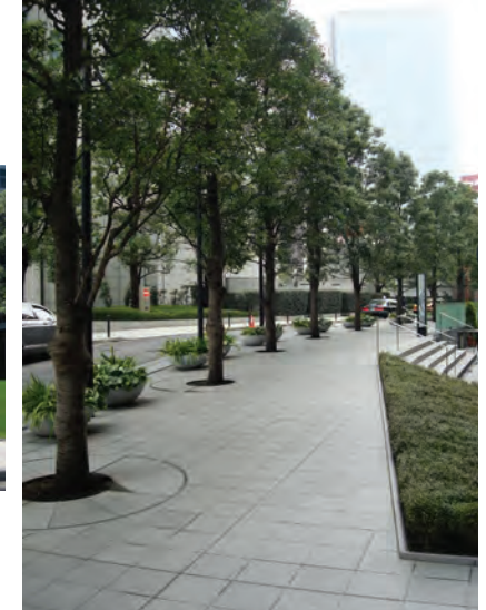
Pavers clearly distinguish the sidewalk from the vehicular route (4.2.3)
