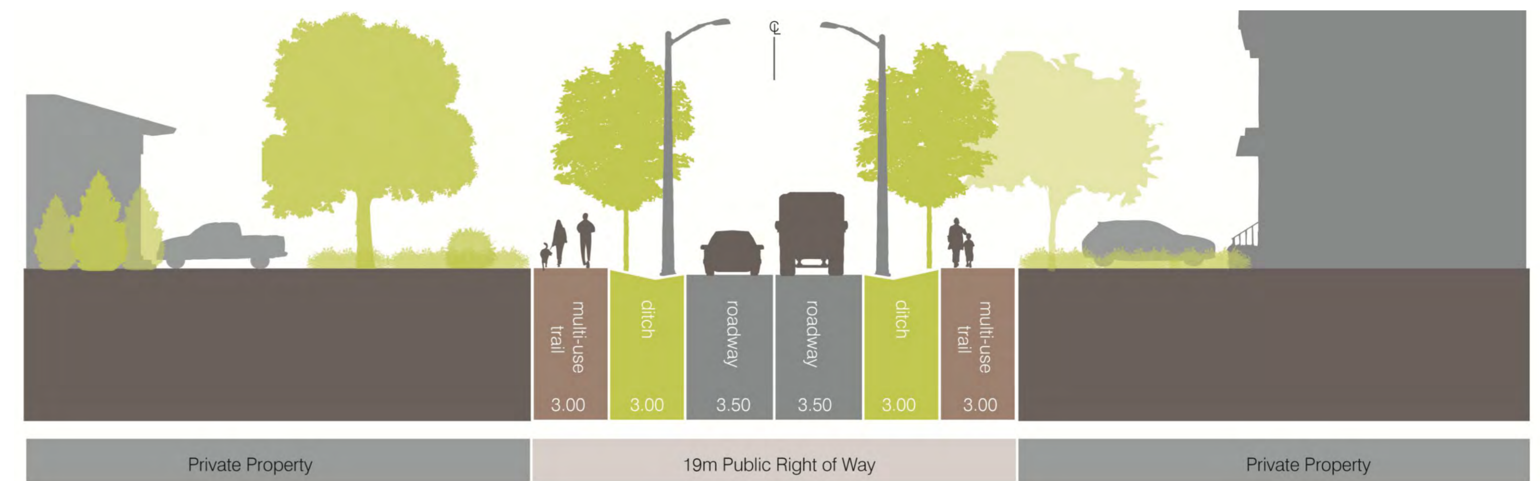
Typical of Rural Corridor with ditches (19m)
