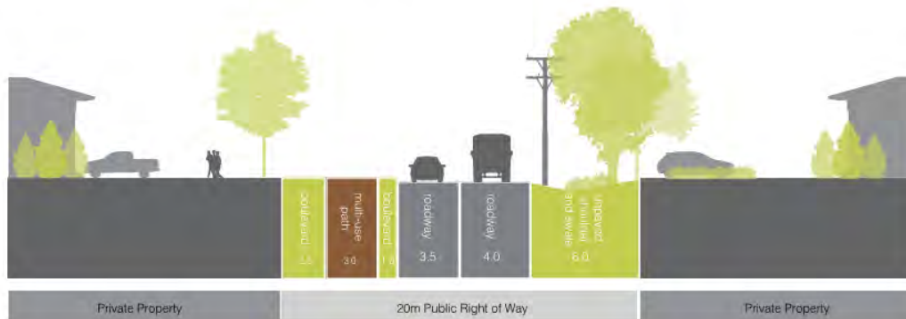
Semi-Urban Roadway with Multi-Use Path 20 metres
