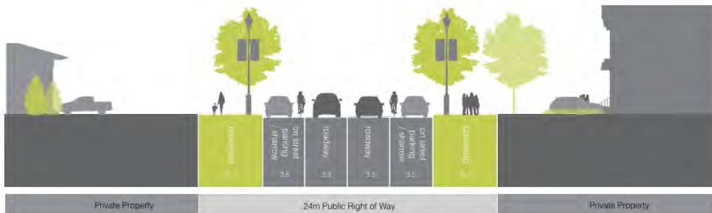
Urban Street On-Street Parking with Sidewalk 24 metres
