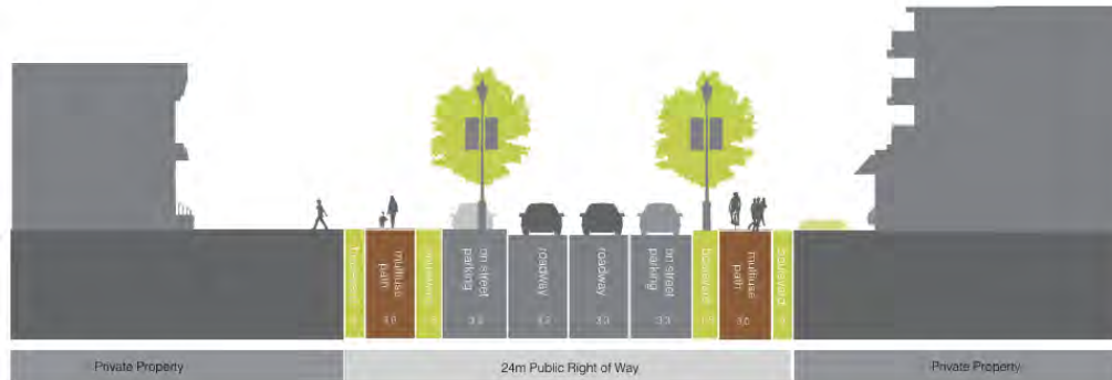
Urban Street Bump Out Parking Lanes with Multi Use Path 24 metres
