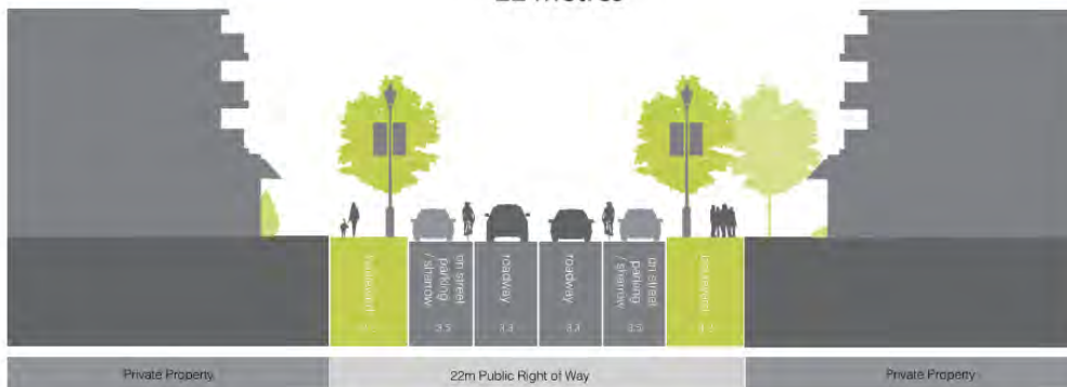
Urban Street On-Street Parking with Sidewalk 22 metres
