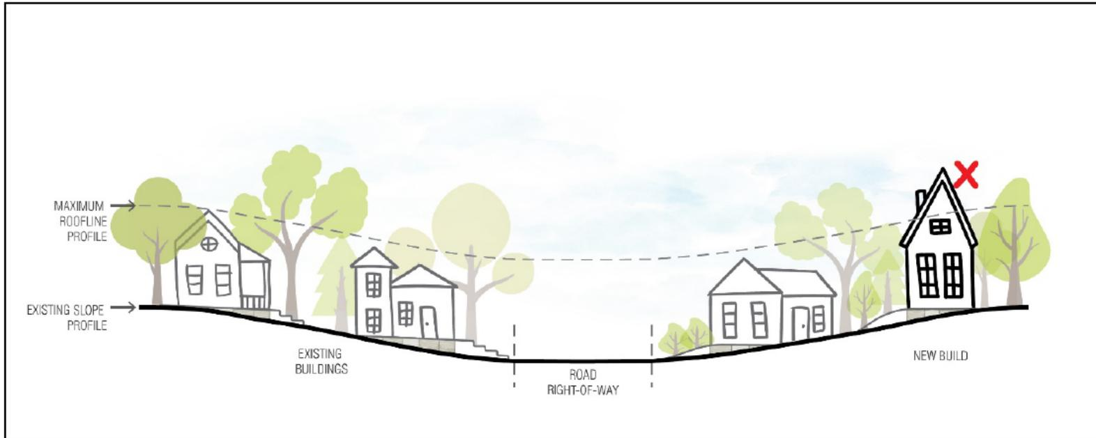
**Figure 32: Building Elevation and Height Following the Topographical Slope**
