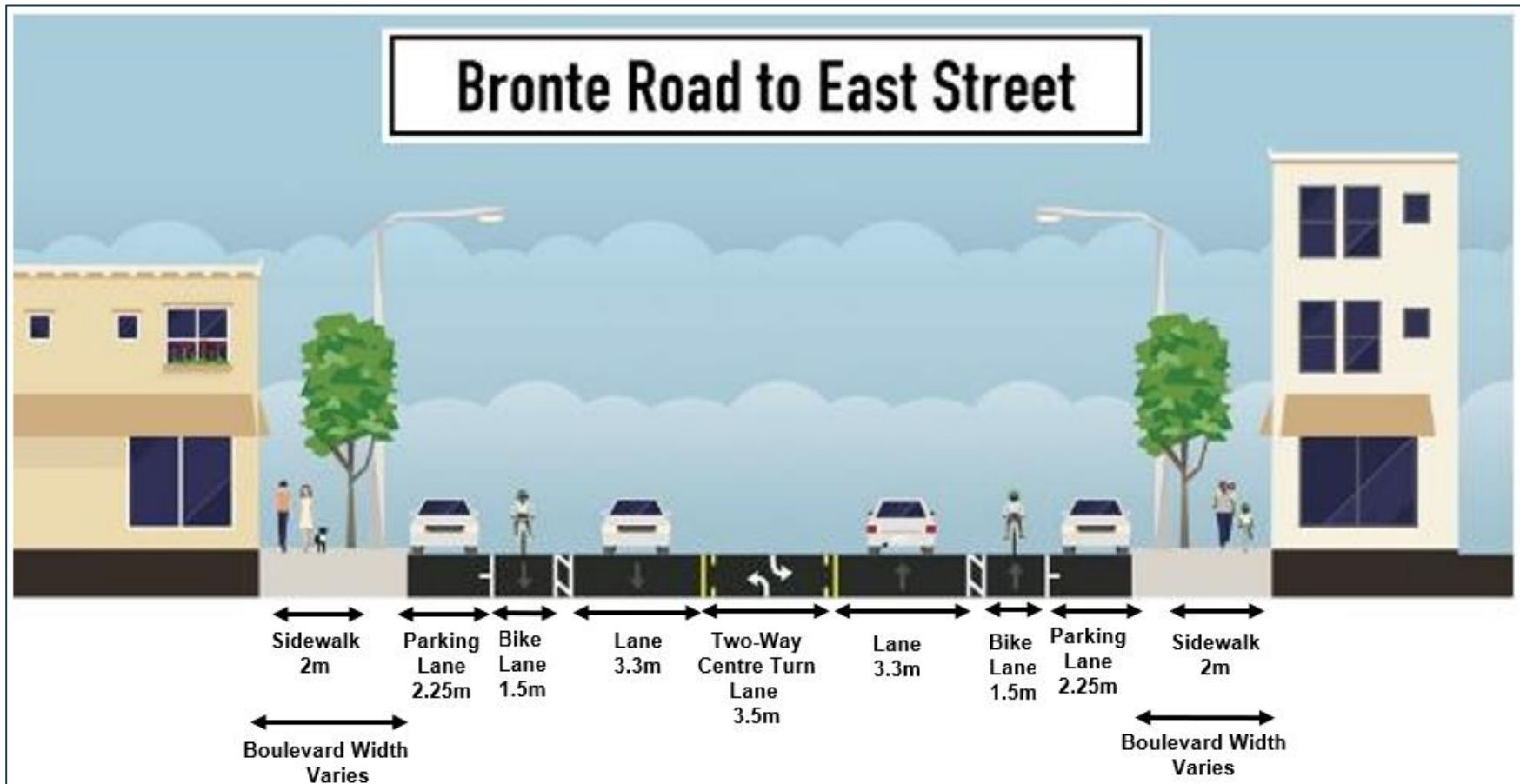
Figure 7-2: Bronte Road to East Street Typical Cross-section (with parking either side or both)
