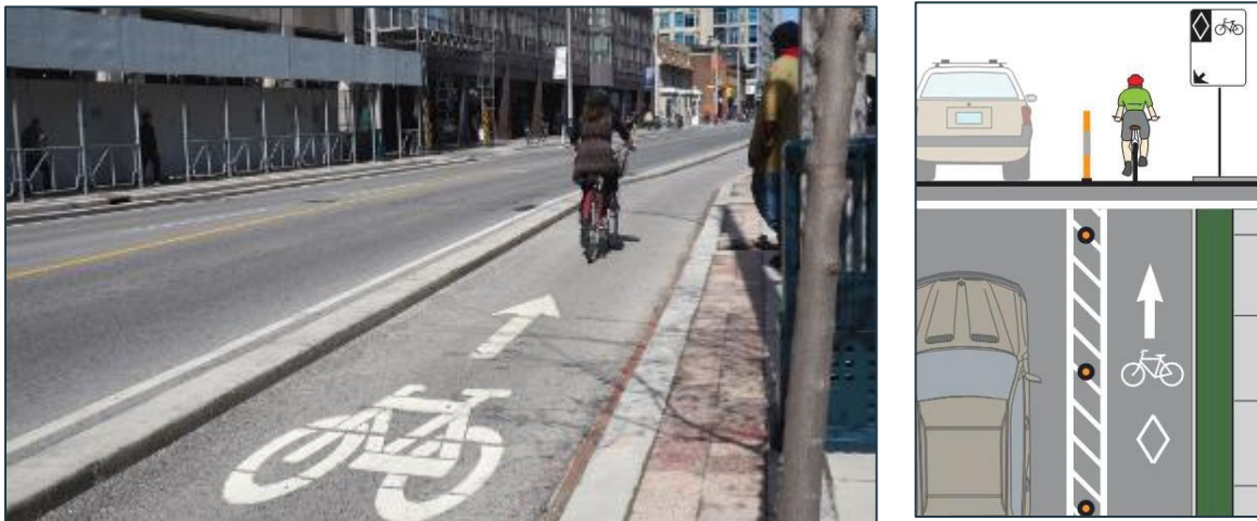
Figure 6-9: Option 2 – 1.5m Separated (Protected) On-Road Bike Lane with Fixed Curbs and Delineators
