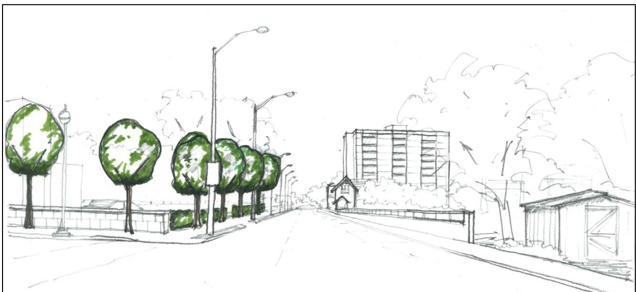
The addition of low, ornamental walls or hedging located on private property (within a planting bed or sod verge) screens parked cars from the pedestrian view and defines the edge of the road allowance.
