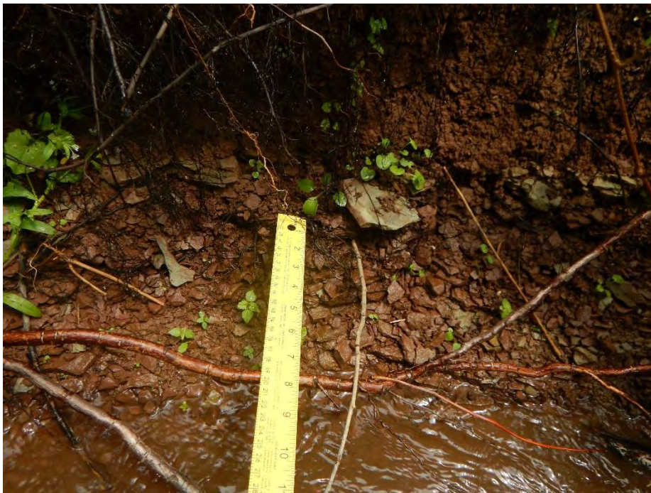
The channel showed evidence of degradation, including the presence of a suspended armour layer consisting of Queenston Shale within the banks, and parent material on the channel bed.
