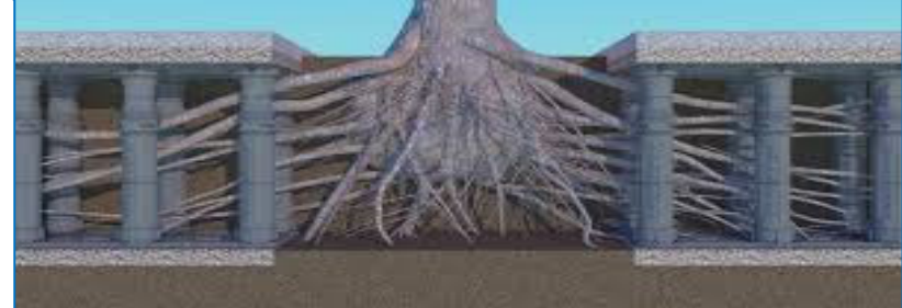
Soil Cell Cross Section
