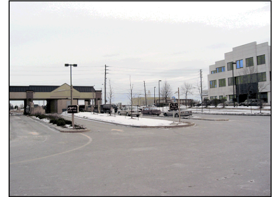
The rear of this drive through facility on Woodbine Ave. in Markham with two restaurants and three stacking lanes illustrates the large maneuvering area required to make the site operate efficiently and safely.
