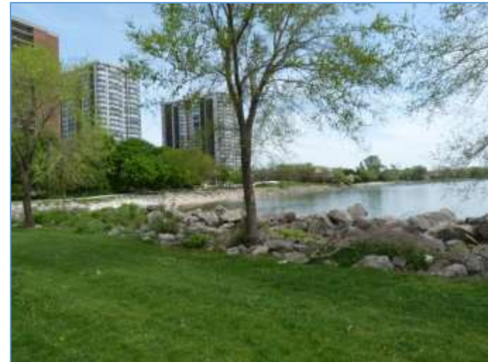
Stone piled along shoreline to prevent erosion presents an opportunity for naturalization
