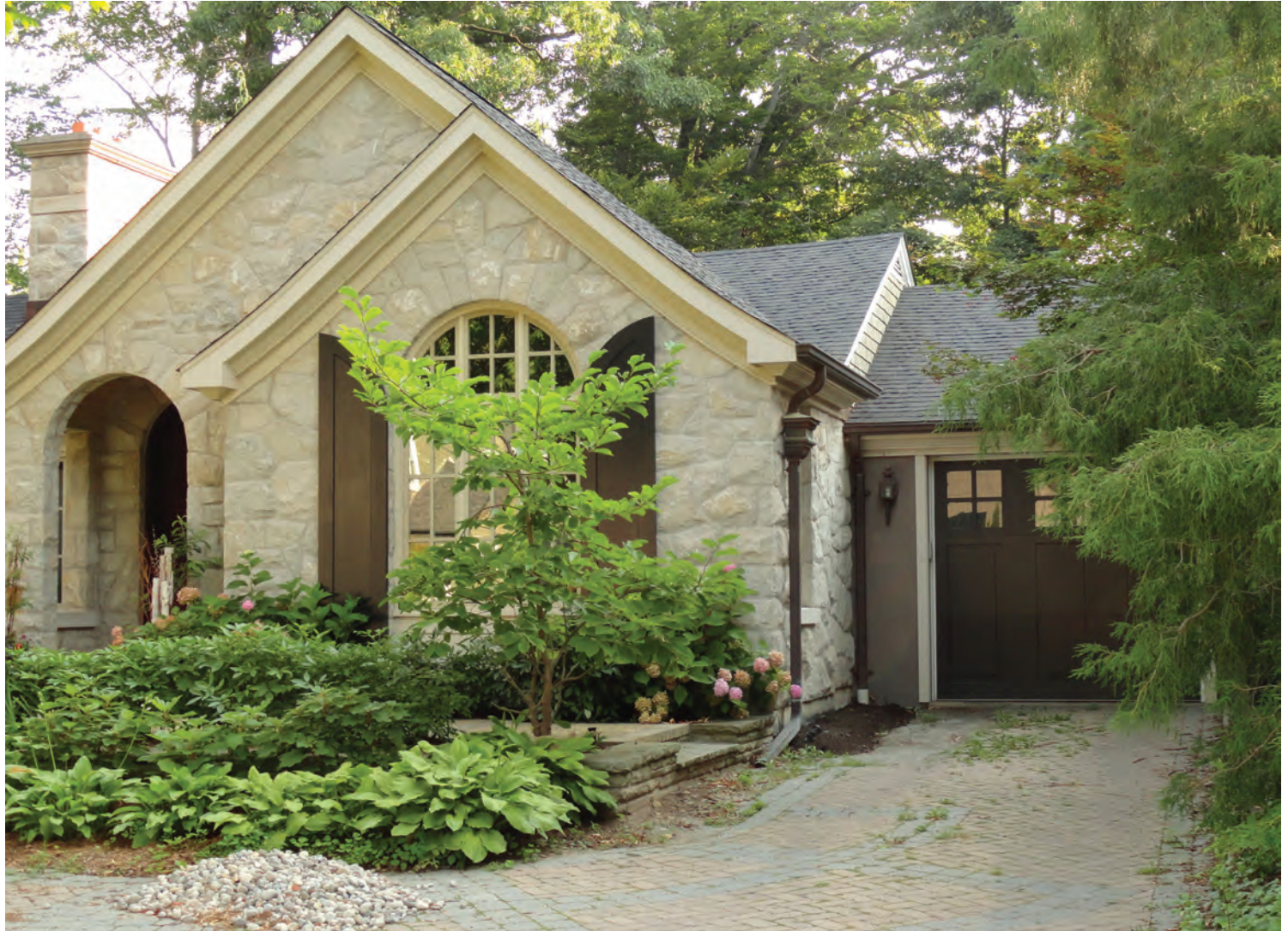
Permeable paving materials can help manage storm water run-off and create a visually softer alternative to commonly used asphalt.
