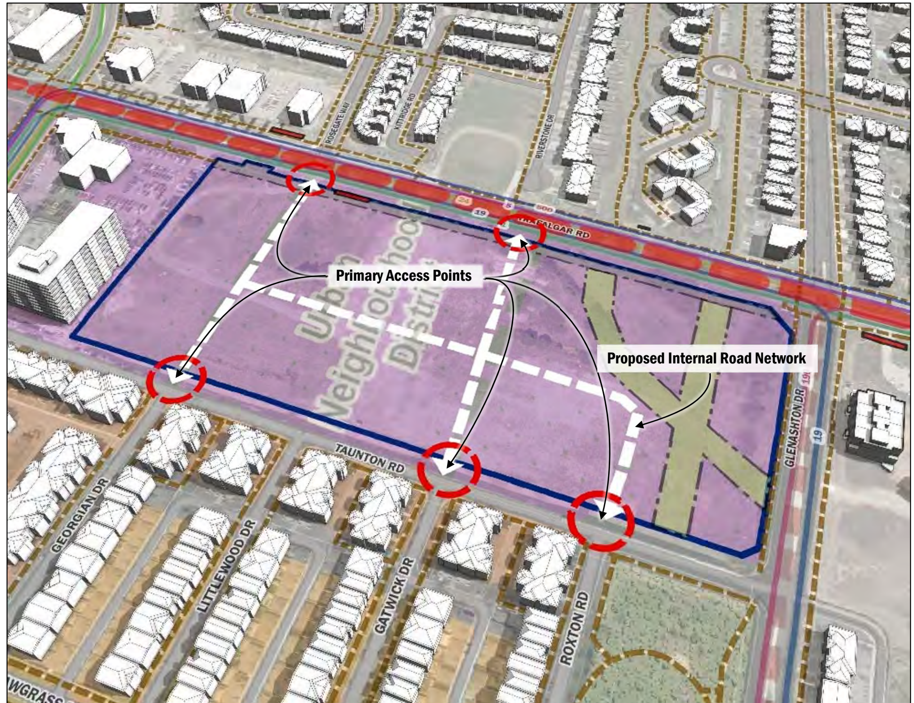
Figure 14 | Internal Road Network
