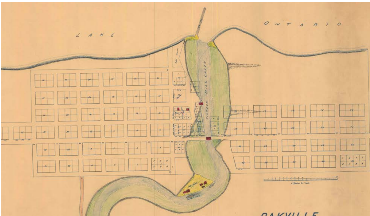
Figure 4-8: Detail of 1833 Castle Plan showing the initial townsite layout, the east breakwater, Chisholm's first shipyard, and several stores and warehouses in red (OHS).
