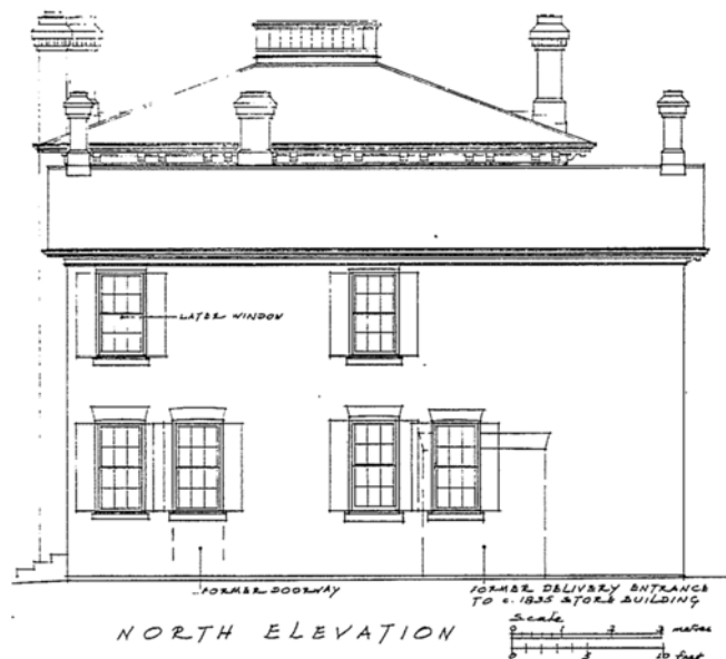
Figure 14: North façade of the Store with notes indicating the historic location of doorways. 89
