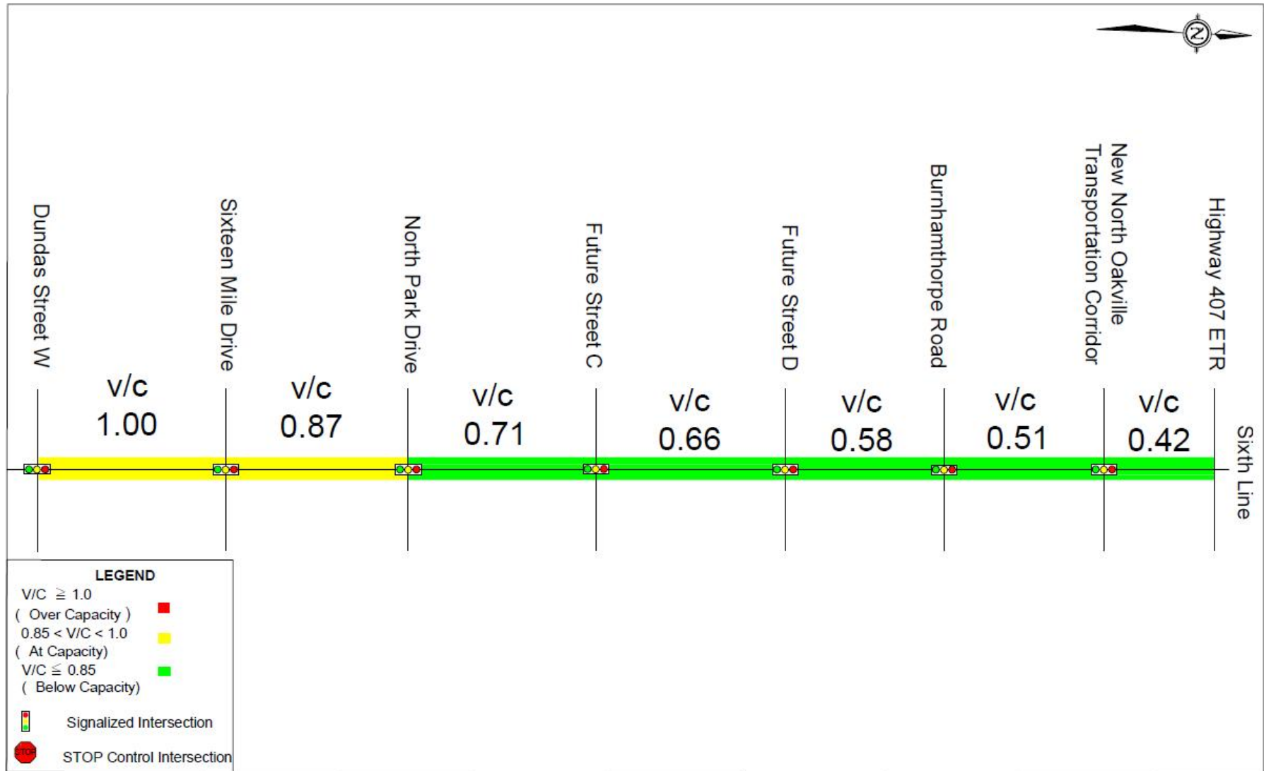
Figure 4-9 Future (2031) PM Peak Hour Mainline Analysis with Improvements (Widening to Four Lanes)
