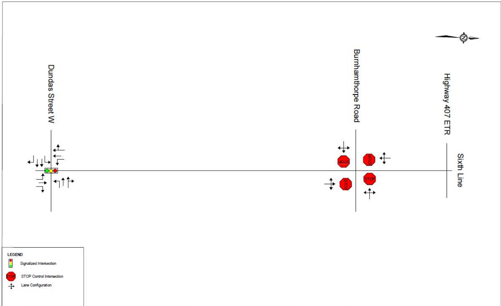
Figure 4-1 Existing (2012) Lane Configuration
