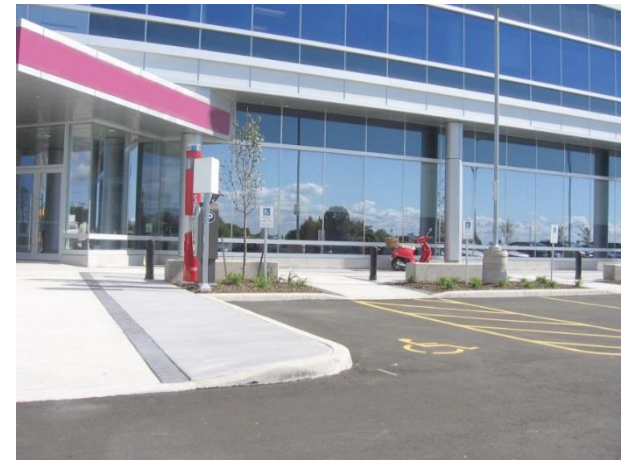
Barrier free parking stalls located close to main entrance providing adequate access to adjacent exterior paths of travel (3.3.8)
