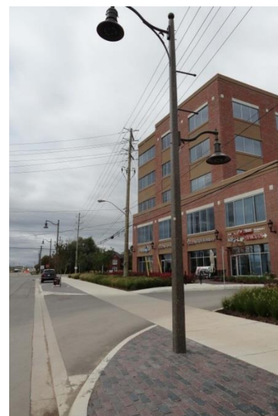
Continuous sidewalk through vehicular entrance (3.2.5)
