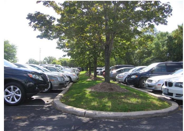
3 m wide continuous parking island breaks up large areas on surface parking and supports healthy tree growth (2.8.3 & 2.8.4)
