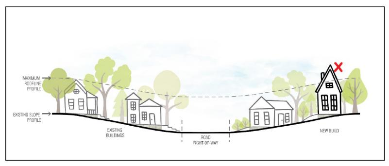
Figure 32: Building Elevation and Height Following the Topographical Slope
