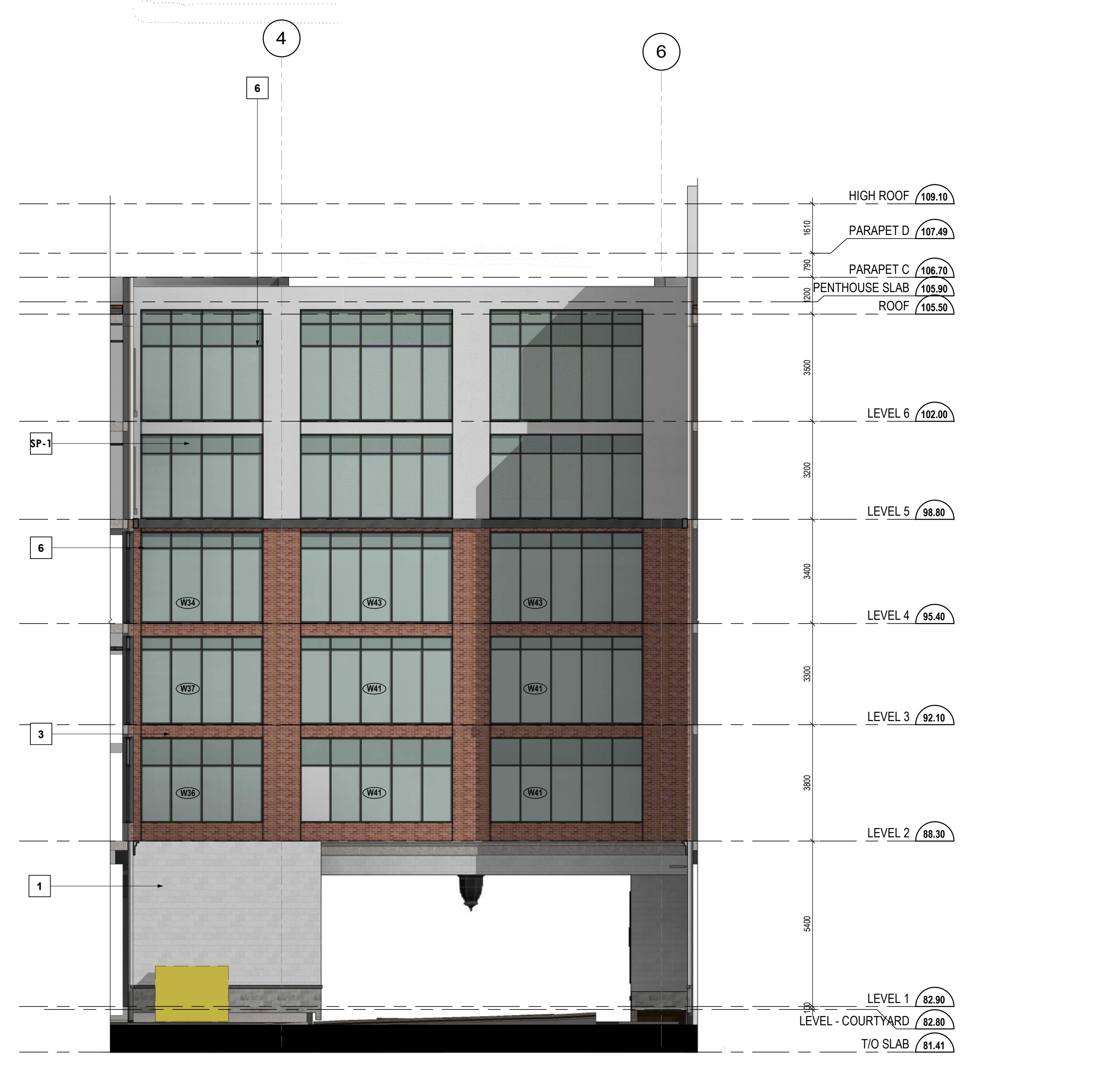
COURTYARD - NORTH ELEVATION 1 SCALE: 1:100 A302
