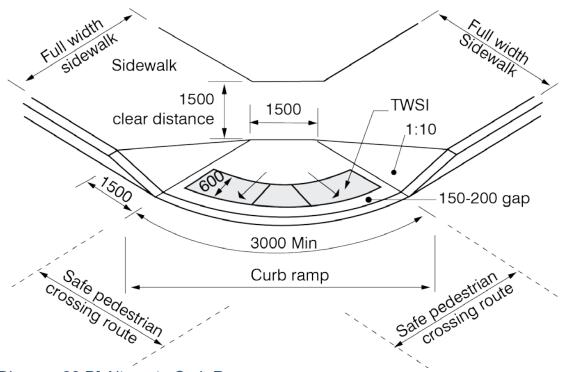
[Diagram 39.D] Alternate Curb Ramp
