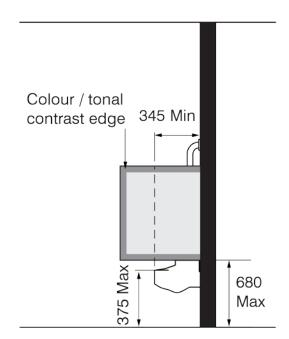
[Diagram 20.D] Accessible Urinal Side Elevation
