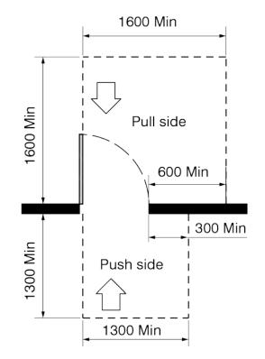
[Diagram 14.D] Latch Side Clearances and Manoeuvring Space
