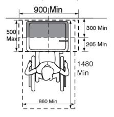
[Diagram 30.D] Knee and Toe Clearance (Plan)
