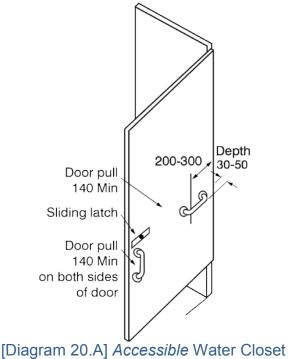
[Diagram 20.A] Accessible Water Closet Stall Door 2. Collapsible coat hooks must be provided, projecting a *max* **50 mm** outward, with a height between **900 mm** and **1200 mm** *AFF*.
