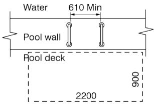
[Diagram 47.D] Transfer Wall Plan View
