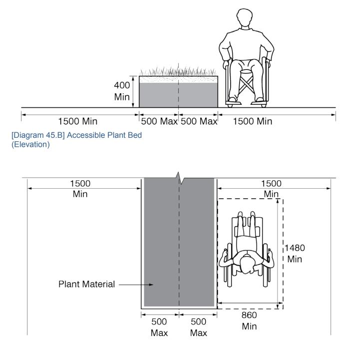
Diagram 45.C] Accessible Plant Bed (Plan)
