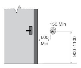
[Diagram 15.C] Circular Power Door Operator (push button)
