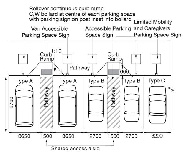
Note: where there is a curb directly in front of the type "A" & "B" barrier-free parking spots a curb ramp will be required at the shared access aisle
