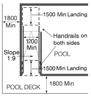
[Diagram 47.A] Submerged Pool Ramp
