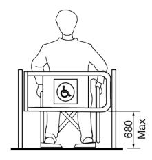
[Diagram 46.B] Accessible Gate in Elevation
