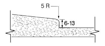
[Diagram 39.A] Curb Ramp Transition at Pavement
