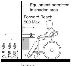
300 Min 205 Min [Diagram 30.C] Knee and Toe Clearance (Elevation)
