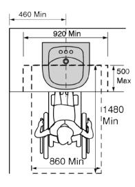
[Diagram 29.F] Sink Floor Plan
