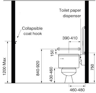
[Diagram 20.D] Accessible Water Closet and Grab Bars Front Elevation
