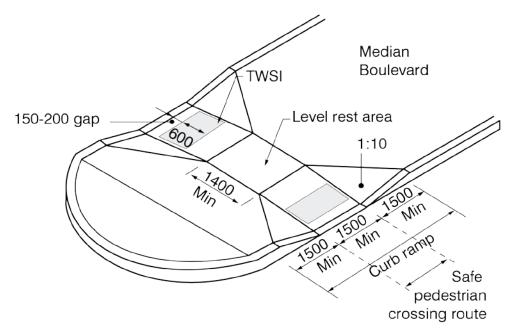
[Diagram 39.F] Curb Ramp at Wide Median Sidewalk Crossing
