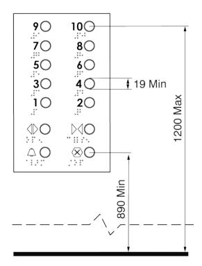
[Diagram 17.B] Elevator Car Control Buttons
