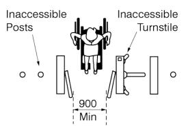
[Diagram 46.C] Accessible Gate in Floor Plan
