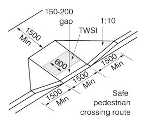
[Diagram 39.B] Curb Ramp at Mid-Block Crossing
