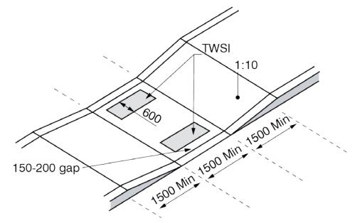
[Diagram 39.E] Curb Ramp at Narrow Sidewalk
