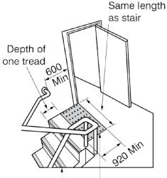
Visual contrast TWSI at top of on top and front stair face of nosing
