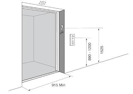
[Diagram 17.A] Elevator Cab and Elevator Lobby
