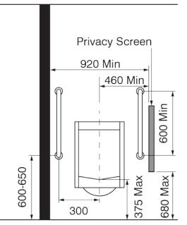
[Diagram 20.C] Accessible Urinal Front Elevation
