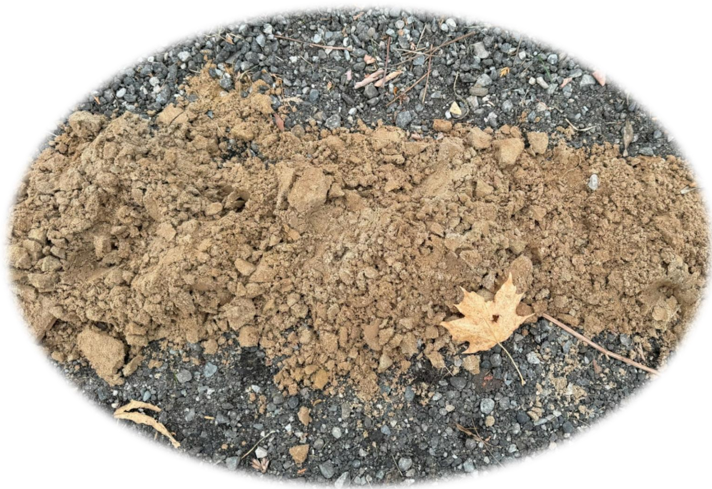
Figure 1: Local Sandy Soils taken from soil probe core during infiltration testing.
