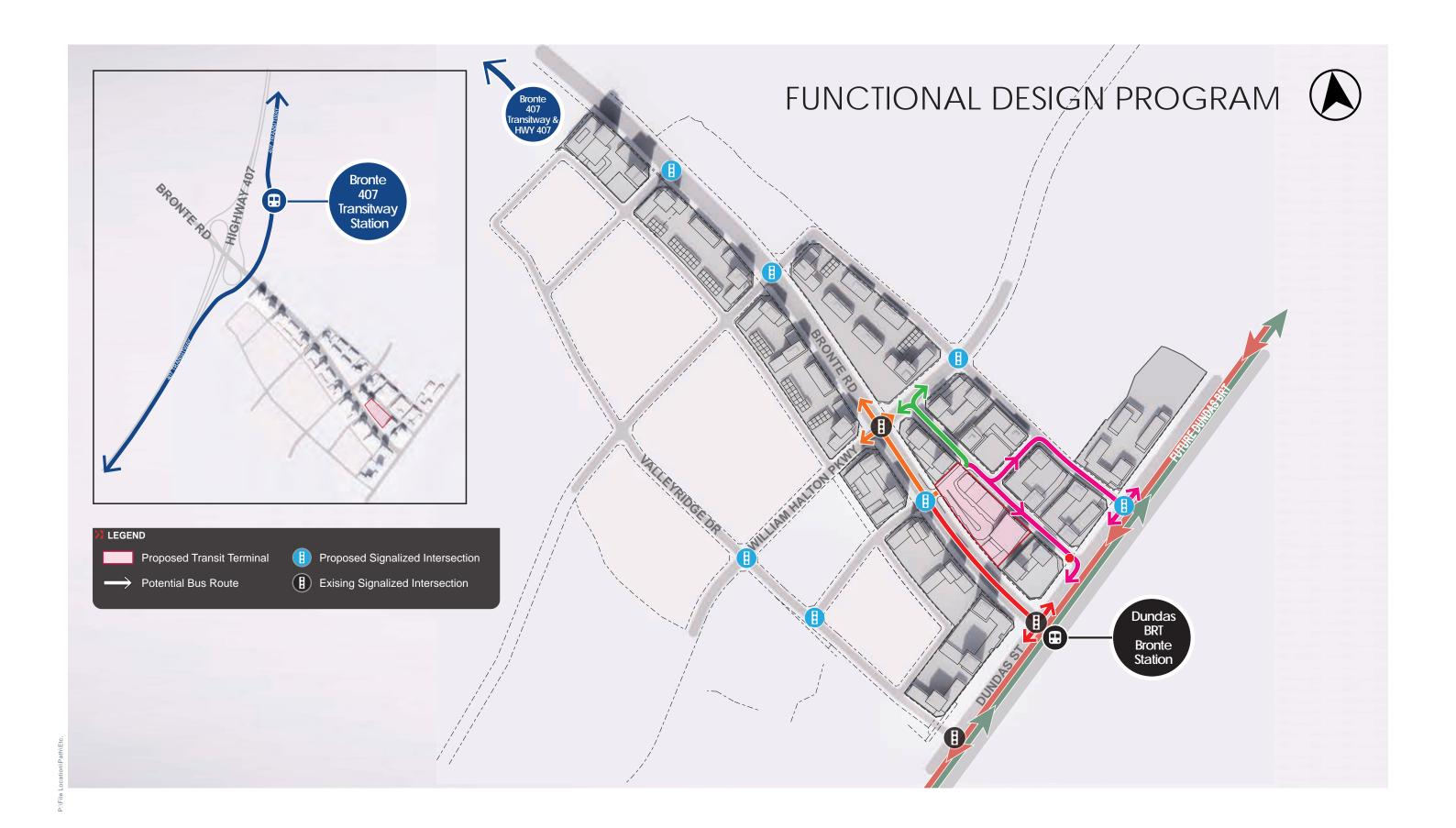
FIGURE 12A PROPOSED PALERMO TRANSIT TERMINAL SERVICE PLAN
