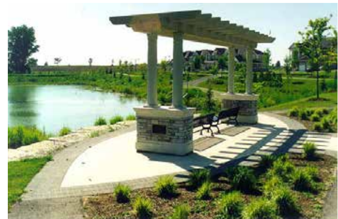
Fig 6.1.1d - Example of a SWM pond lookout amenity with decorative paving, bench seating and shade structure, situated at a visually prominent location within the neighbourhood and aligned with the SWM pond multi-use trail / maintenance access.
