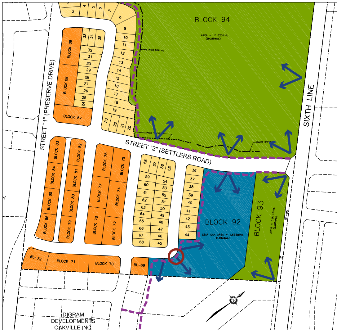
Fig 6.1.1b - Conceptual SWM pond layout showing intended location of trail / service access road and views.
