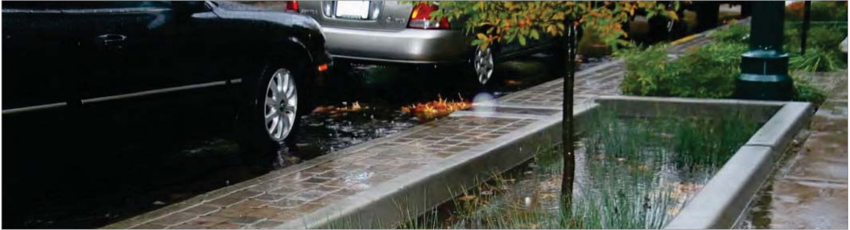
On-site stormwater retention areas and infiltration areas reduce the requirement for end-of pipe stormwater infrastructure (NOUDG)
