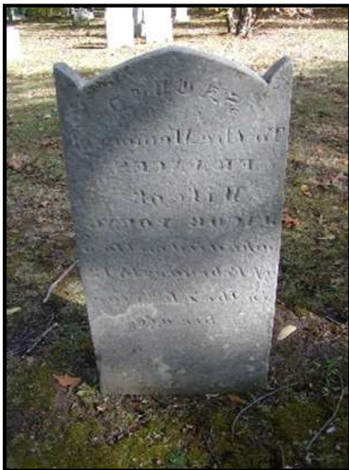
Figure 39: The limestone markers of Jacob and Frances Young, after restoration in November 2017, and in November 2021. Note the extensive weathering and loss of detail in just four years. 255
