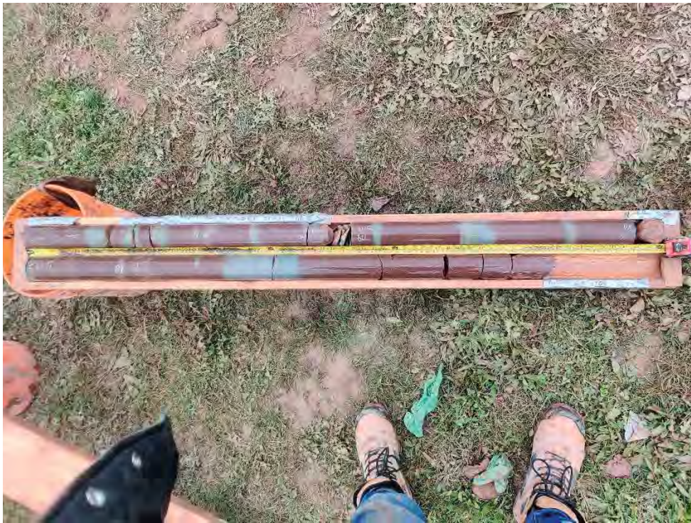
BH209 Rock Core Run 7 & Run 8 (57.5' to 66.6') / RQD 86% to 88% Good Quality
