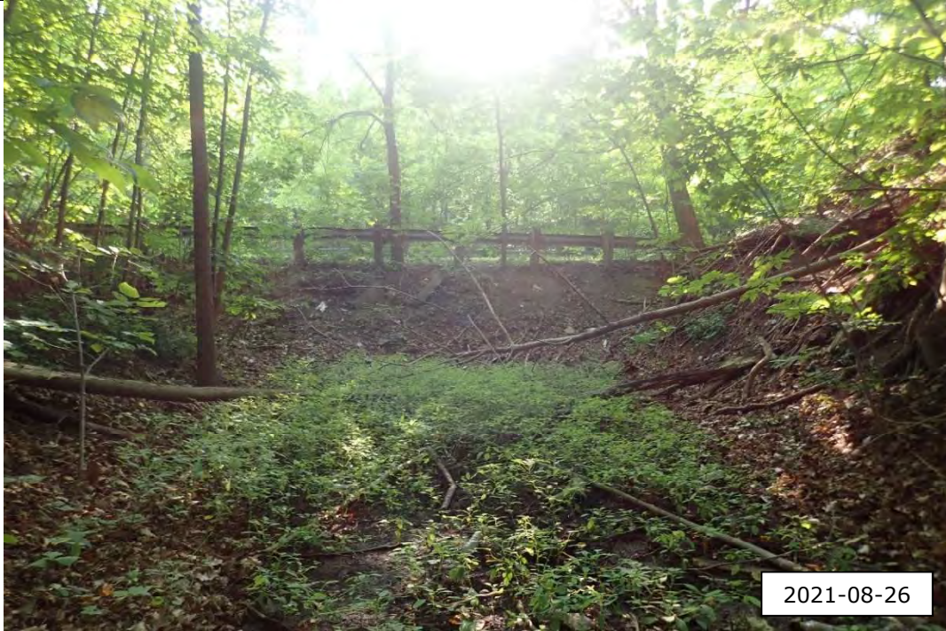
Downstream view of the watercourse. The reach was dry at the time of assessment. Average bankfull width and depth were 3.08 m and 0.24 m, respectively.
