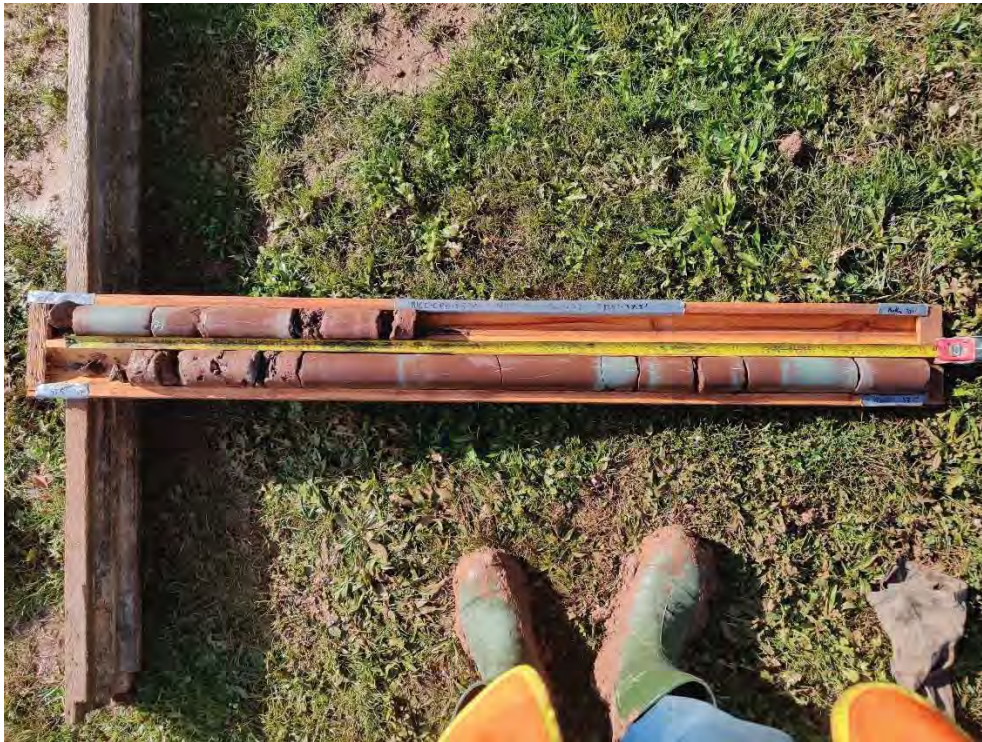
BH209 Rock Core Run 1 & Run 2 (30.5' to 37.5') / RQD 46% to 59% Poor to Fair Quality
