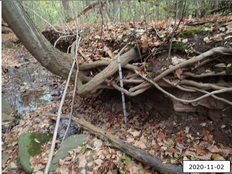
Mature tree roots were commonly exposed on the banks. Substrate was coarse and consisted of platy pebbles and cobbles derived from the shale material.
