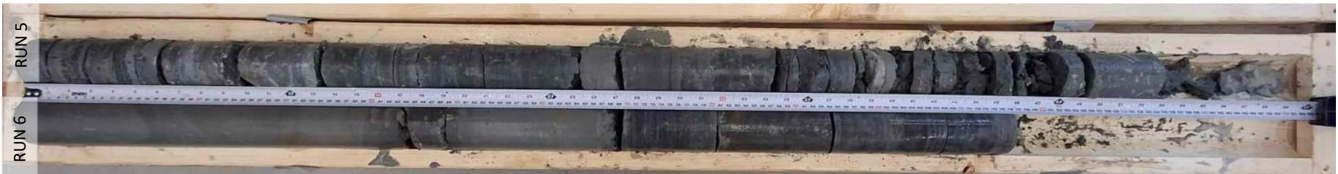
Borehole MW-333: Run 5 (10.66 to 11.94 m) and Run 6 (11.94 to 13.13 m)
