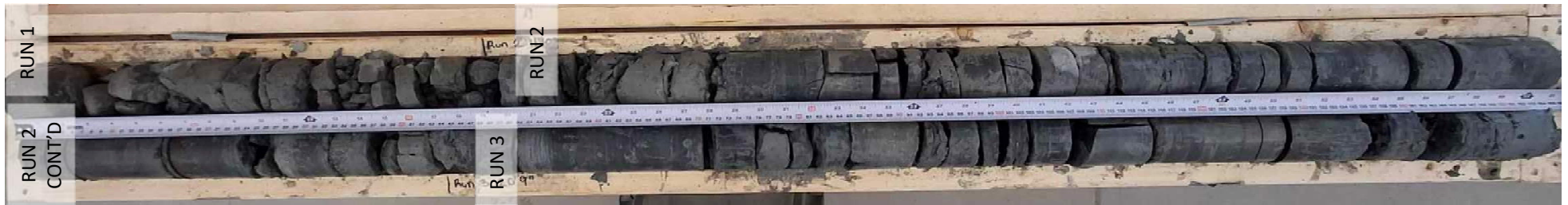
Borehole MW-337: Run 1 (2.84 to 3.61 m), Run 2 (3.61 to 4.78 m) and Run 3 (4.78 to 6.32 m)
