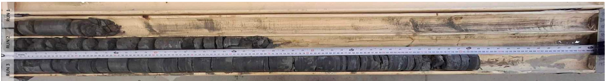
Borehole BH-401: Run 1 (2.74 to 3.20 m), Run 2 (3.20 to 4.72 m) and Run 3 (4.27 to 5.95 m)
