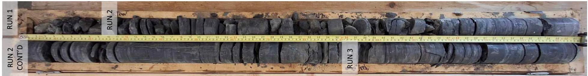
Borehole MW-334: Run 1 (3.20 to 4.75 m), Run 2 (4.75 to 6.27 m) and Run 3 (6.27 to 7.79 m)
