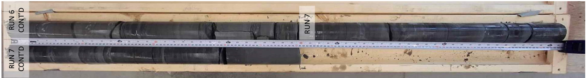
Borehole BH-404: Run 6 (12.42 to 13.84 m) and Run 7 (13.84 to 15.27 m)
