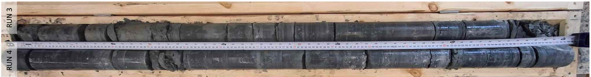
Borehole MW-332D: Run 3 (7.62 to 9.14 m) and Run 4 (9.14 to 10.72 m)
