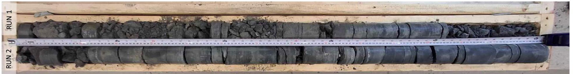
Borehole BH-403: Run 1 (3.20 to 4.34 m) and Run 2 (4.34 to 5.94 m)
