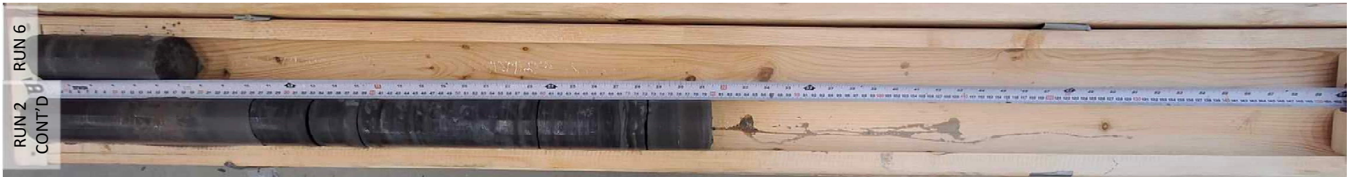
Borehole MW-339: Run 6 (10.69 to 12.34 m) and Run 7 (12.34 to 13.13 m)
