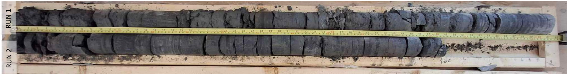
Borehole MW-333: Run 1 (4.90 to 6.44 m) and Run 2 (6.44 to 7.77 m)
