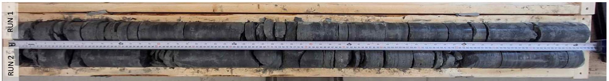
Borehole MW-338: Run 1 (3.55 to 5.00 m) and Run 2 (5.00 to 6.40 m)
