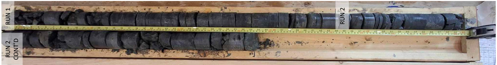
Borehole MW-332D: Run 1 (4.58 to 6.10 m) and Run 2 (6.10 to 7.62 m)
