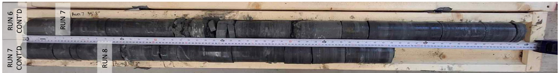
Borehole MW-337: Run 6 (9.17 to 10.87 m), Run 7 (10.87 to 12.27 m) and Run 8 (12.27 to 13.11 m)
