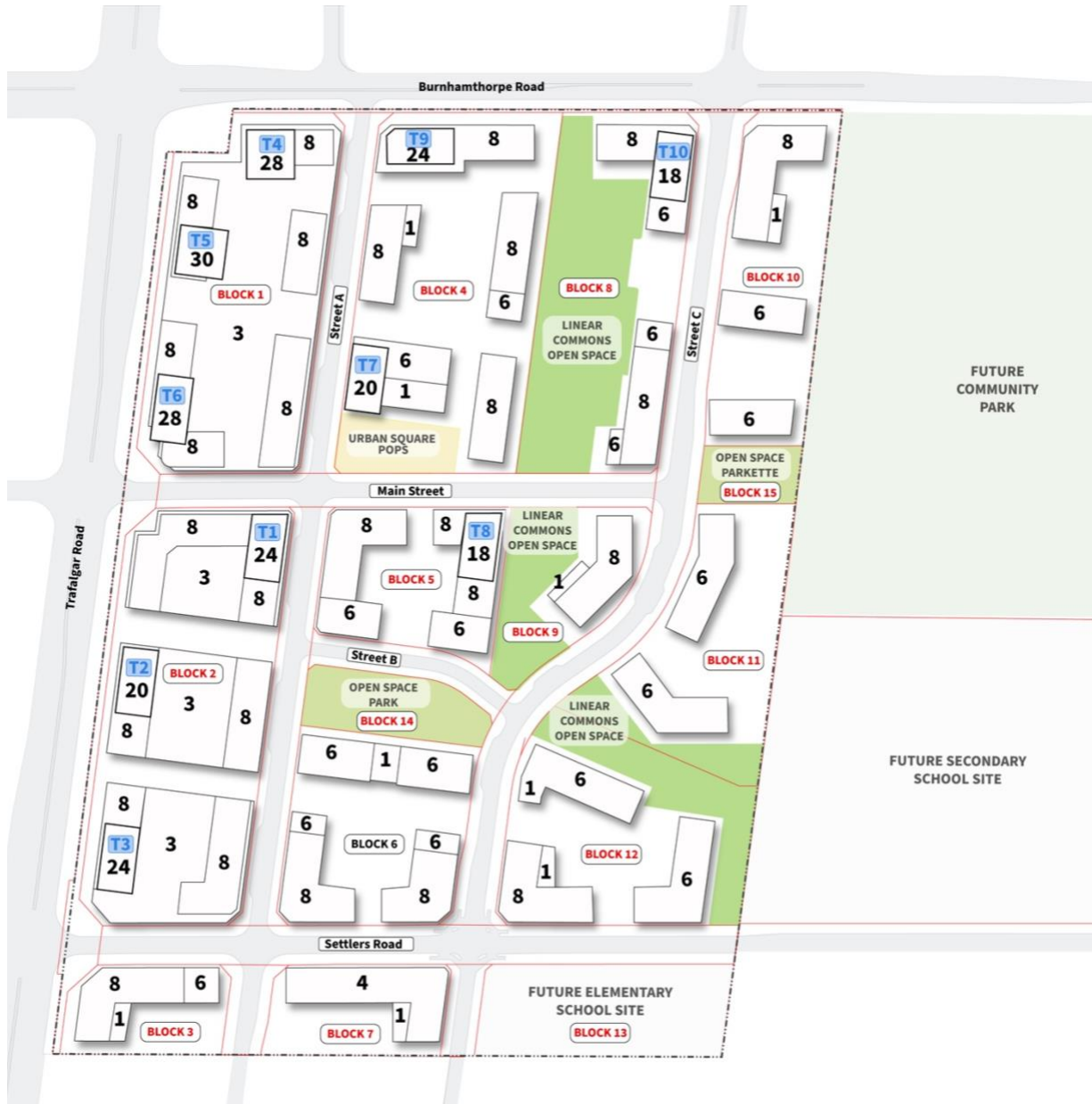
Annotated site plan of the Proposed Development with tower numbering and building heights.
