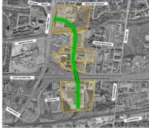
Improvement A4 – Along section of North Service Road and extending north of diversion channel creating a new intersection with Trafalgar Road
