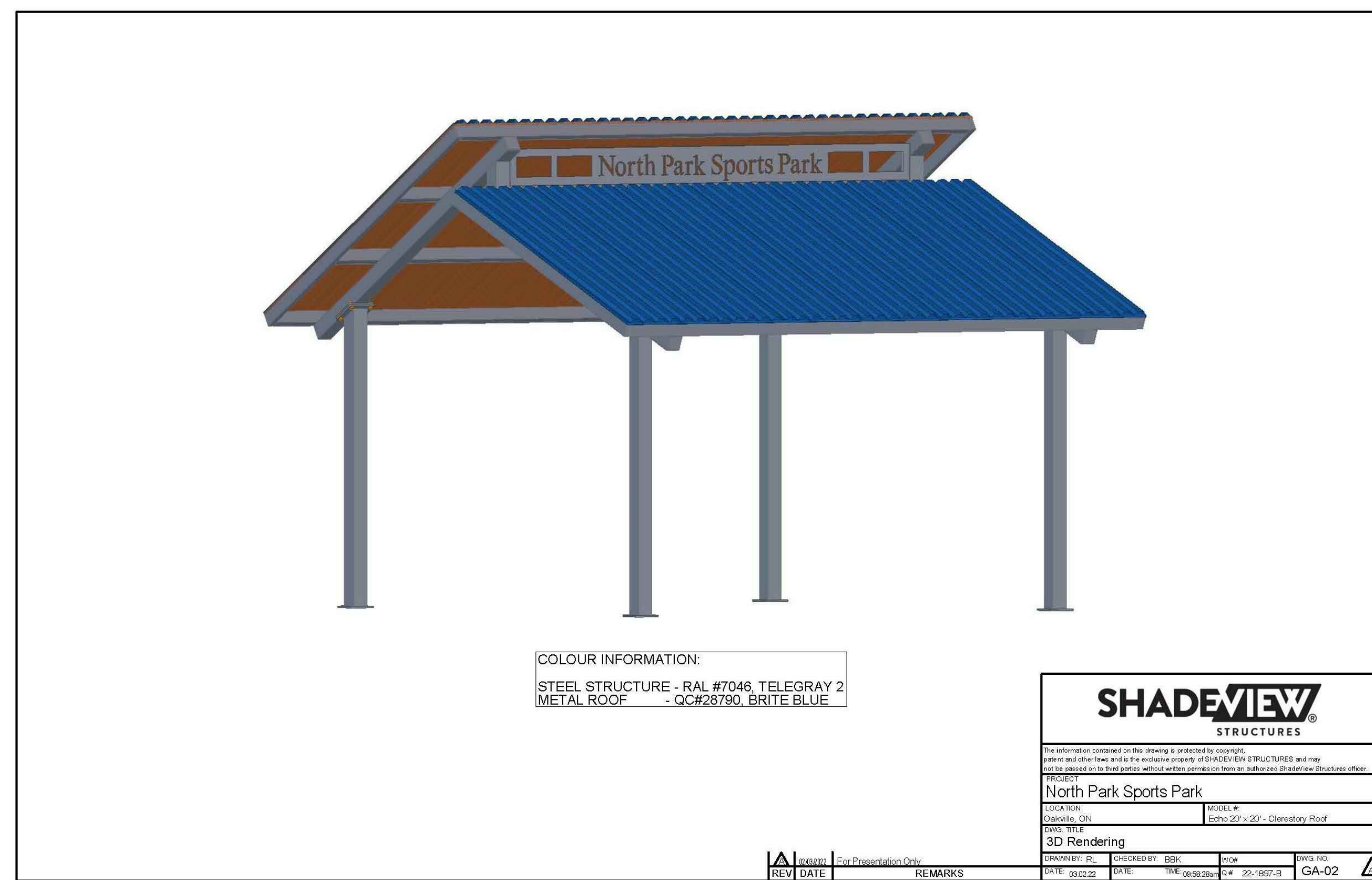
3 MANUFACTURERS SPECIFICATIONS SHADE STRUCTURE - TYPE 2 BY SHADEVIEW (MODEL XXX) OR APPROVED EQUAL
