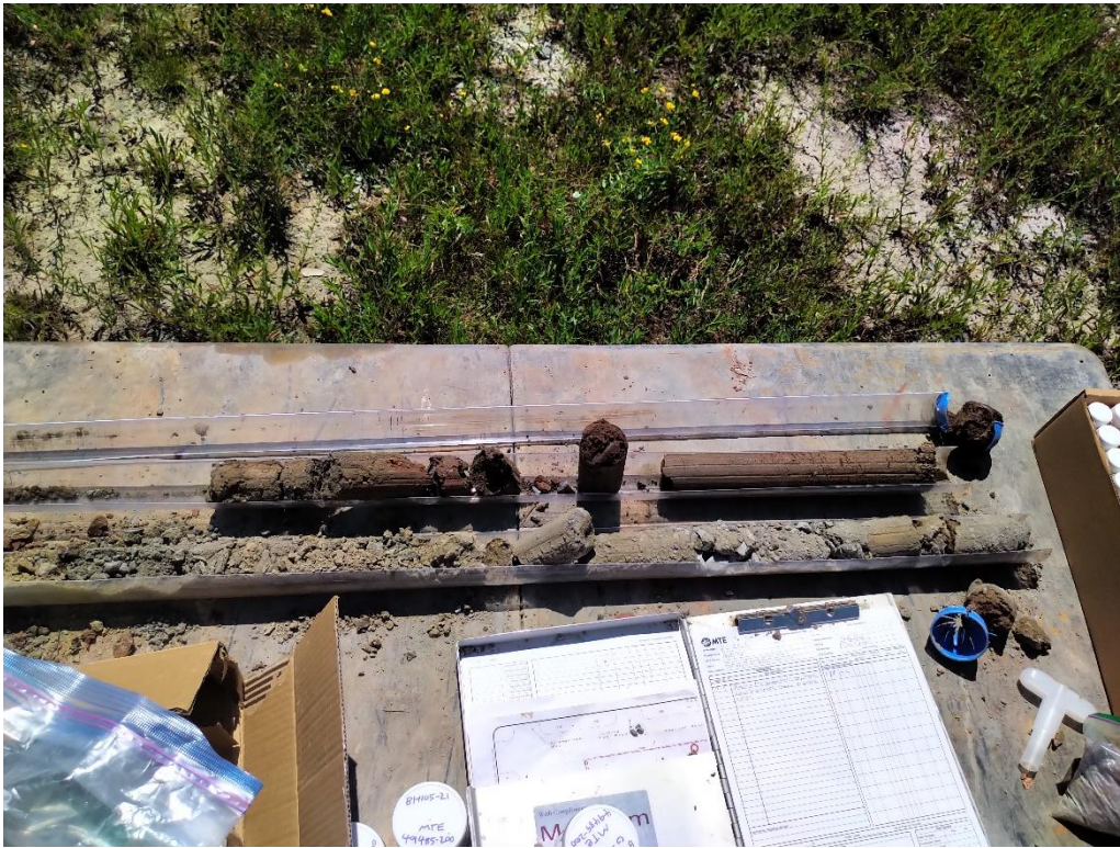
Photograph No. 5 – View of the general soil stratigraphy observed on the Site, including a clayey silt fill over a native clayey silt.
