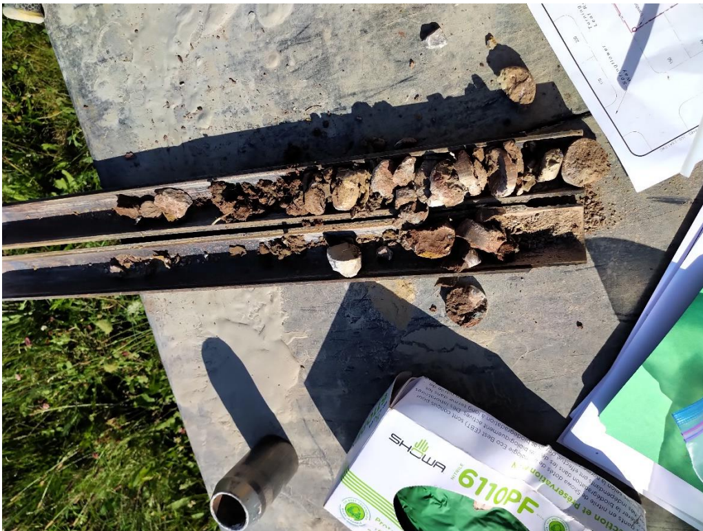
Photograph No. 4 – View of the fill material at borehole BH102-21.
