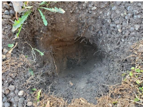
Photo 12: Sample undisturbed test pit with aggregate overburden
