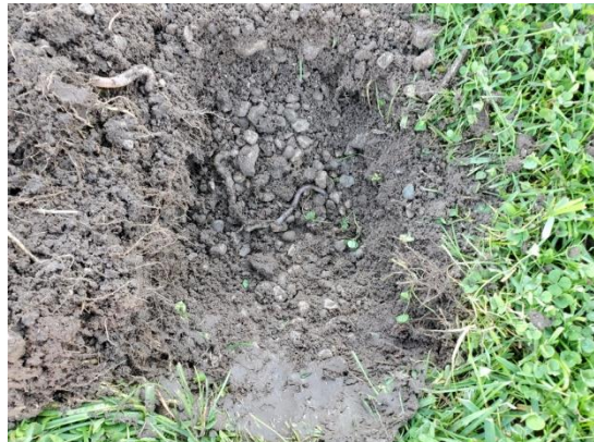
Photo 12: Sample undisturbed test pit with aggregate overburden
