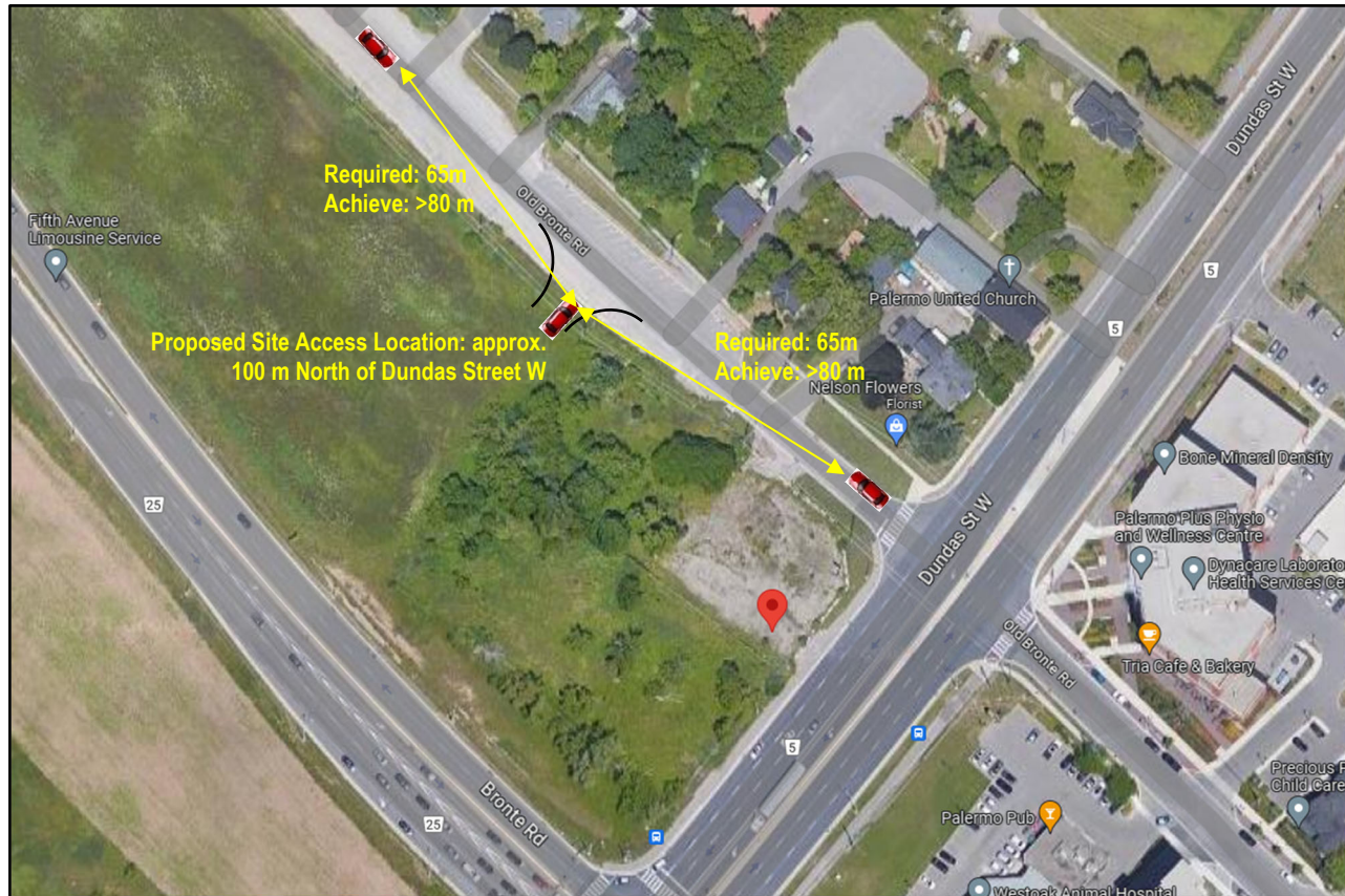
Figure 19 – Site Access Stopping Sight Distance
