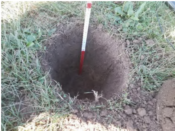
Plate 17: Test pit showing buried A-horizon. Approximately 25 cm of construction fill (Lot 2) overlaying 30 cm of A-horizon (Lot 1) overlaying B-horizon (Lot 2) (sterile subsoil).
