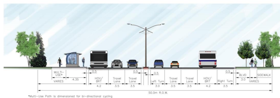
Exhibit ES-3: Typical Intersection Cross-Section with Right-Turn and Left-Turn Lanes
