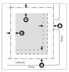
The black circles are letters corresponding to the applicable yard in the regulations table. The shaded area represents the potential building envelope remaining once minimum yards are removed.
