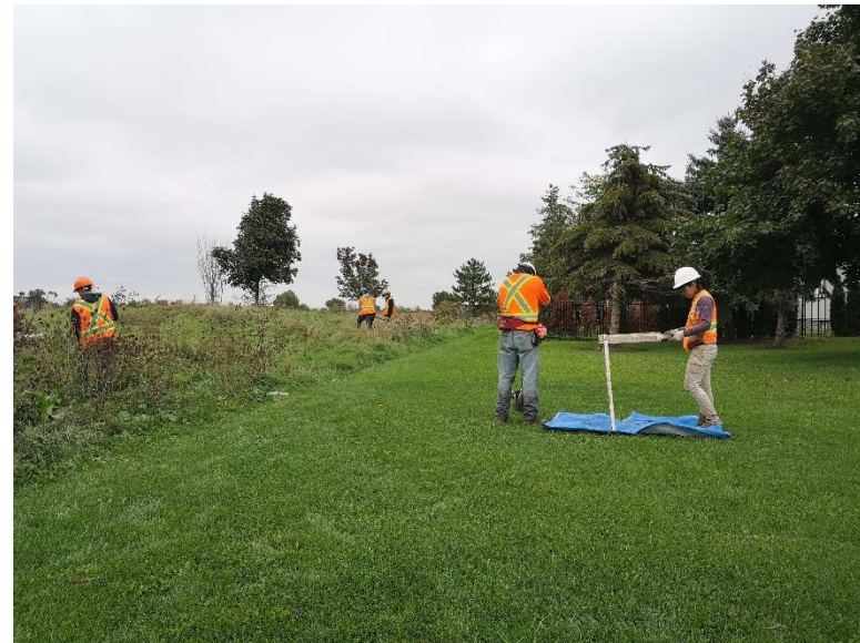
Image 12: View of test pit survey conducted at 10-metre intervals.
