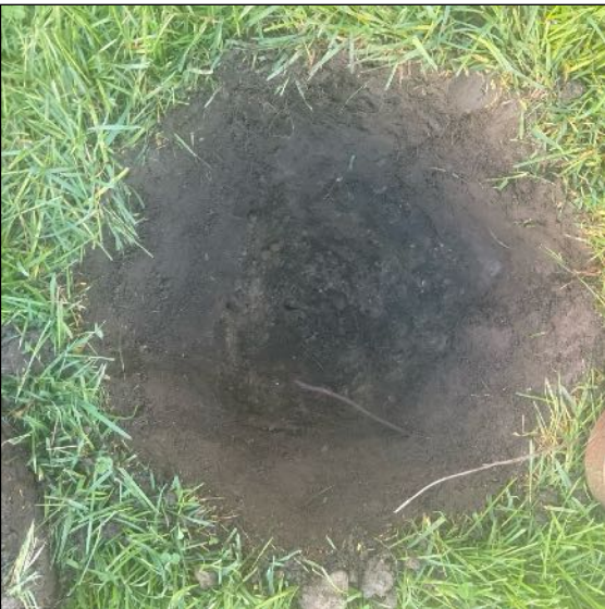
Image 7: Sample Test Pit showing subsoil.
