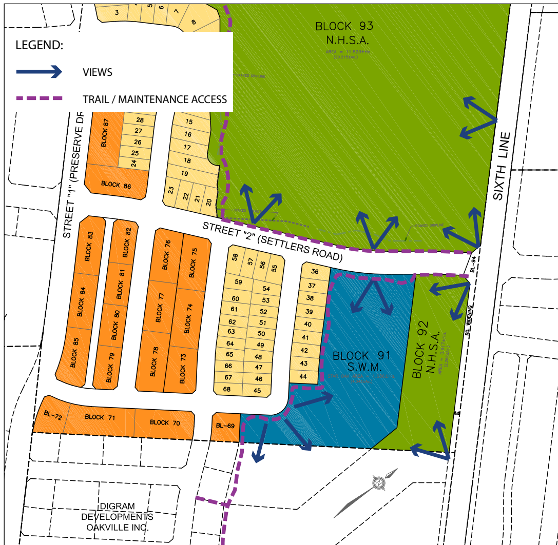
Fig 6.1.1a - Conceptual SWM pond layout showing intended location of trail / service access road and views.
