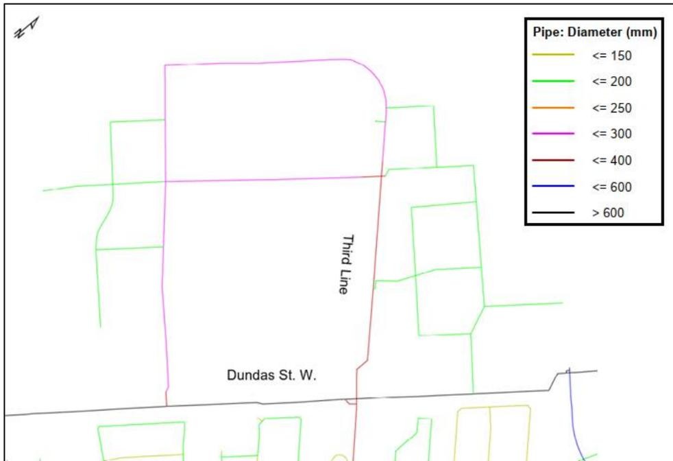
**Figure 3 - New Watermains Proposed in the Study Area with Pipe Diameter**
