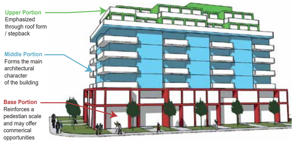
Fig. 3.2.5b - Mixed Use/Apartment buildings should be designed to establish distinct base, middle and upper portions
