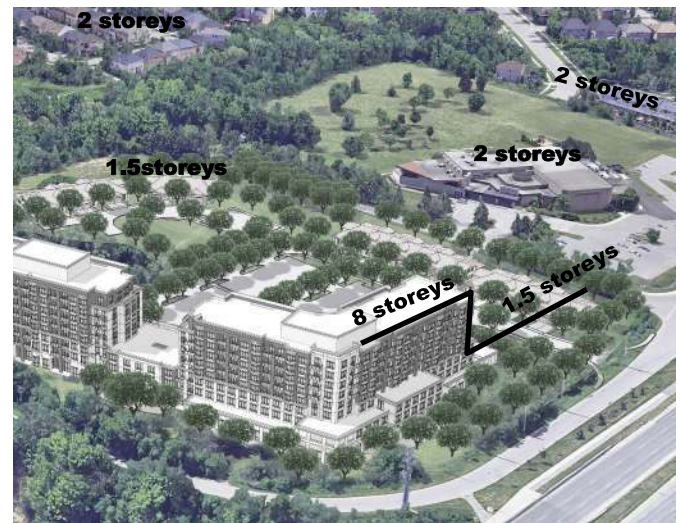
The above graphic illustrates how building heights transition from 8 storeys to 2 storeys with the lower building heights located in proximity to the St. Volodymyr Cultural Centre and existing low rise residential communities.
