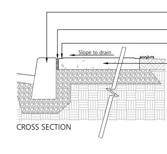
Concrete Curb (By Others) 20mm fiberboard control joint at curbs & walls
