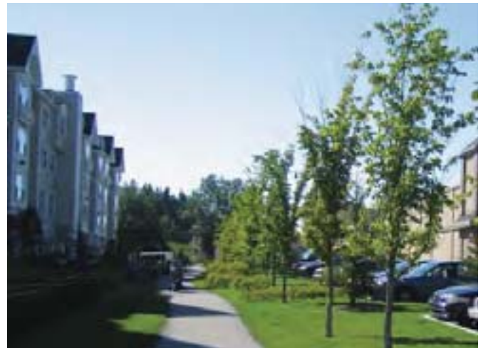
Photo 3.149: Where neighbouring properties have adjacent surface parking lots, a coordinated planting strip of 3.0 metres should be provided between the parking lots to allow sufficient area for parking lot edge treatments, drainage, access, vegetation, fencing and snow storage.
