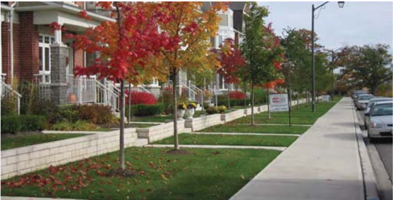
Photo 3.108: Residential sidewalks can align the roadway (bottom photograph) or be set back from the roadway with a landscaped boulevard (above photograph).
