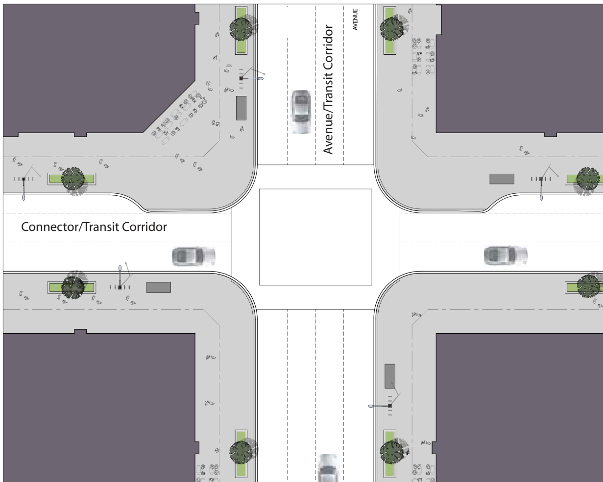
Figure 4.37: Typical Intersection of an Avenue/Transit Corridor and a Connector/Transit Corridor in the Urban Core.
