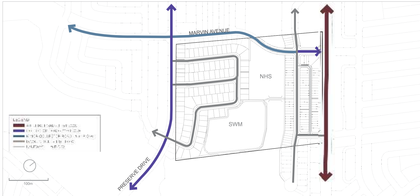
Fig. 4.3 - Road Hierarchy Plan for Argo West Morrison Creek within the surrounding community.
