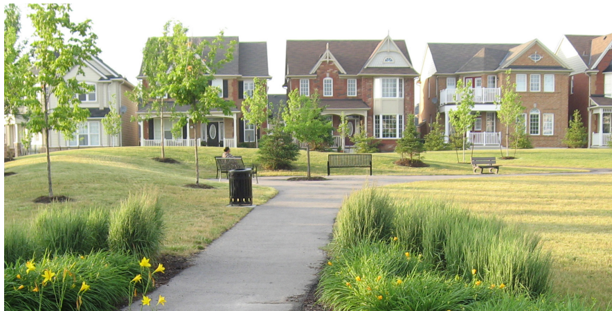
Fig. 7.8.6 - Image example of park facing dwellings oriented to front onto the park, with wide porches that results in informal monitoring of the park and its activities
