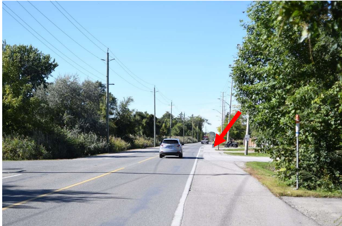
Exhibit 6-45: Stopping Sight Distance – South of Access (Looking Northbound from a point 105 m south of the access)
