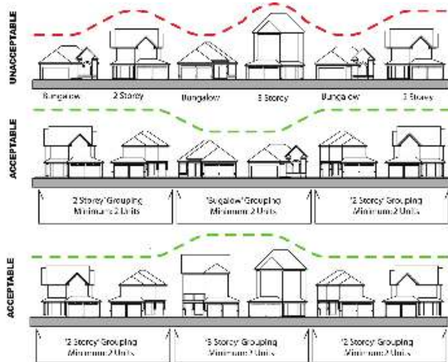
Fig. 7.3b - Diagram illustrating streetscape massing objectives
