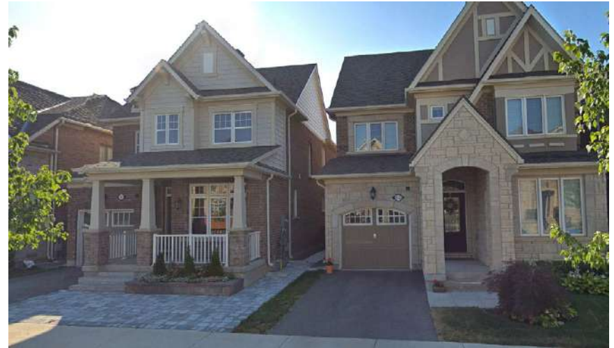
Fig. 6.3.2d - Image example of attached garages integrated into the main massing of the dwelling, behind the porch projection.
