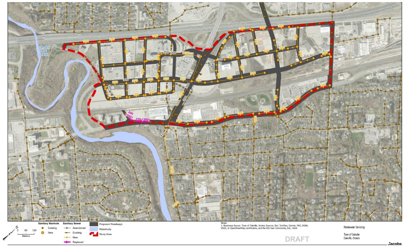
Figure 2-2. Wastewater Servicing Map
